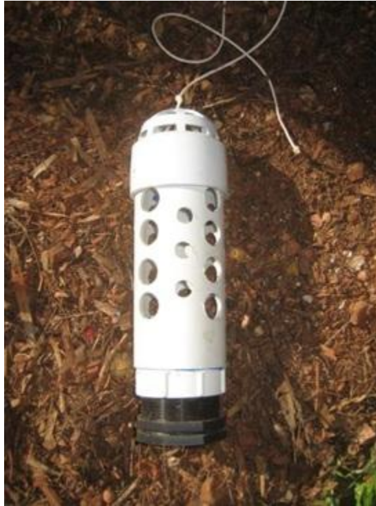
Figure 4. Troglifauna trap used during Phase 2 of the survey which is similar but slightly longer than traps used during Phase 1.
